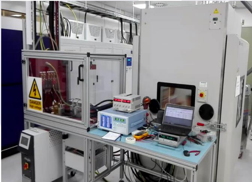
IPU operating with motor under the condition DC450V/AC450Arms
